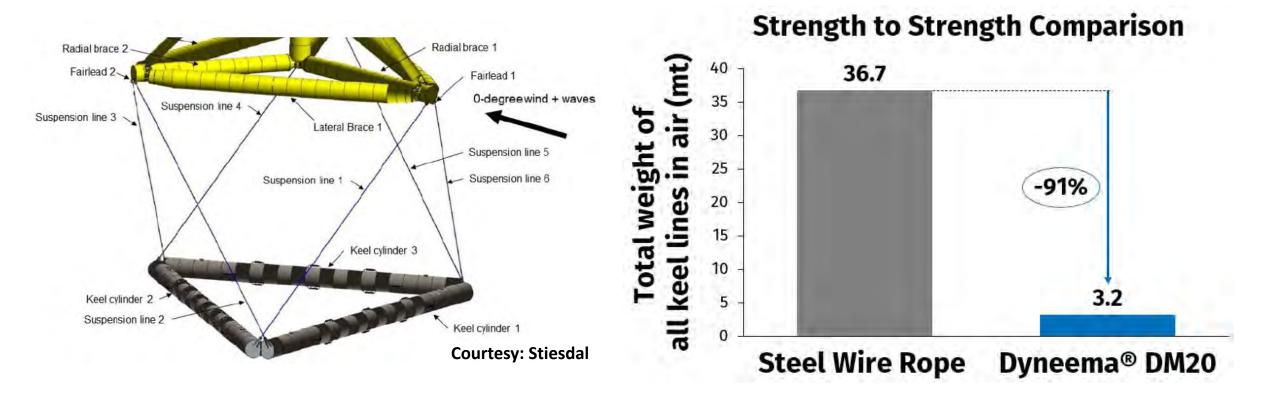
• When submerged, Dyneema<sup>®</sup> is neutrally buoyant – saving 30+ mt of extra buoyancy
