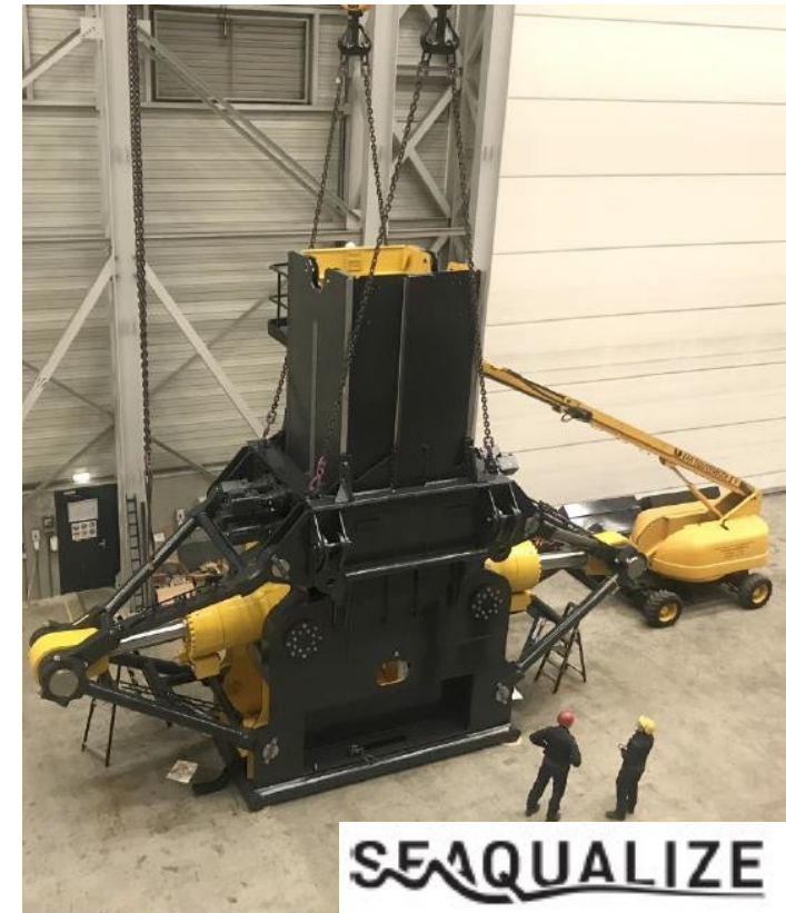
Seaqualize tool In-hook Balanced Heave Compensation
