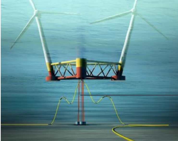
Tension leg or catenary mooring systems for minimal environmental footprint
